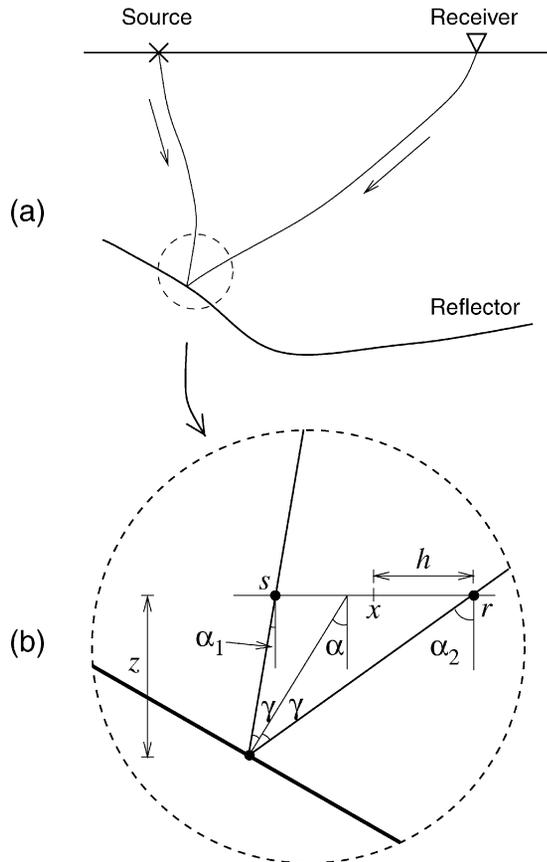
FIG. A-1. Specular energy propagates towards the reflection point as it is downward-continued during migration. In general, the velocity of the overburden may be complex (a); however, the velocity should be smooth in the vicinity of the reflection point (b).
