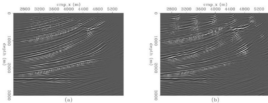
FIG. 5. Migrated images produced with data having a fully-sampled shot axis (a), and a very sparsely sampled shot axis (b).
