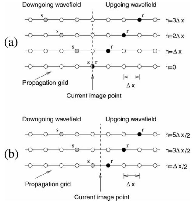
FIG. 2. Midpoint-offset sampling during migration. Panel (a) shows imaging offsets with  $\Delta h = \Delta x$  based on equation (4) alone. Panel (b) shows the additional offsets that are imaged with  $\Delta h = \Delta x/2$ . The midpoints in this panel lie between propagation grid nodes.
