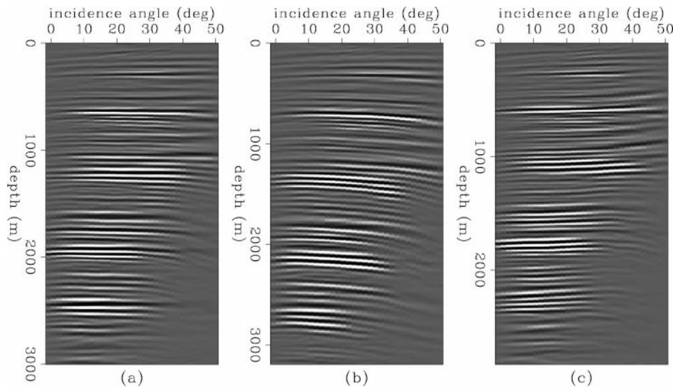
FIG. 4. Angle-domain common-image gathers corresponding to  $x = 4000$  m. Panels (a), (b), and (c) were migrated with velocity models that were correct, too high, and too low, respectively.
