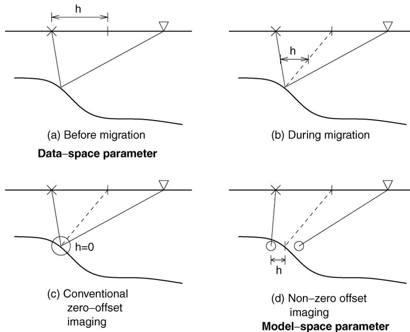
FIG. 1. Illustration of how the effective offset of specular energy changes as the wavefield is downward continued into the earth. Panels show offset before (a), during (b), and after (c, d) migration.
