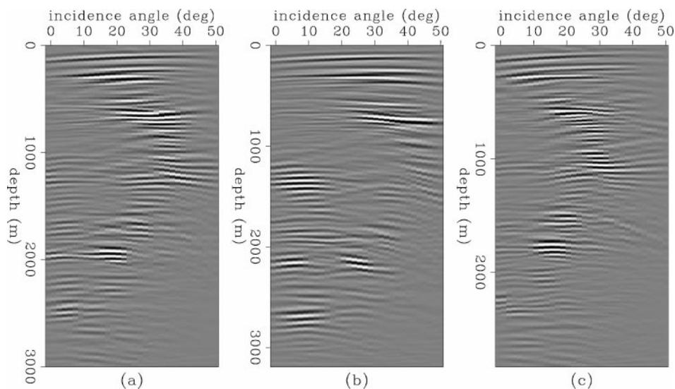
FIG. 7. Poorly illuminated angle-domain common-image gathers corresponding to  $x = 4000$  m. Panels (a), (b), and (c) were migrated with velocity models that were correct, 6% too high, and 6% too low, respectively.
