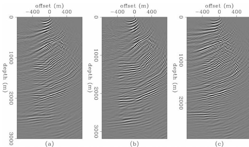
FIG. 6. Poorly illuminated offset-domain common-image gathers corresponding to  $x = 4000$  m. Panels (a), (b), and (c) were migrated with velocity models that were correct, 6% too high, and 6% too low, respectively. Shot spacing was 500 m, instead of 25 m as in Figure 3.
