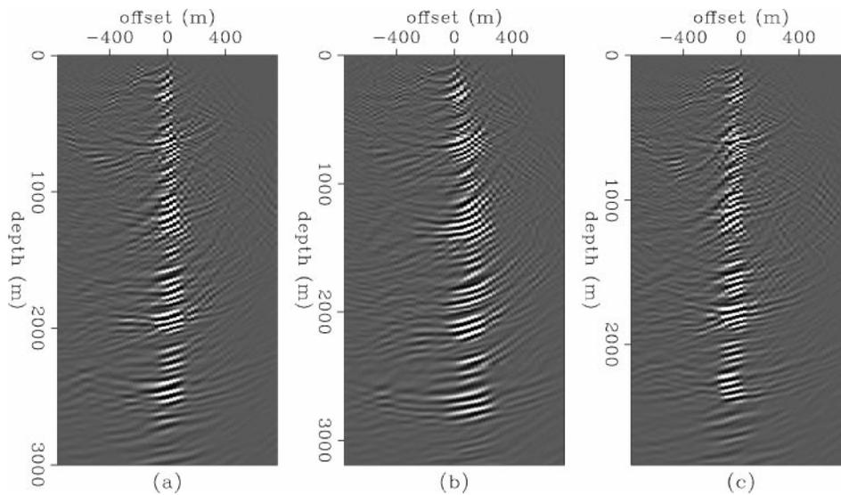
FIG. 3. Offset-domain common-image gathers corresponding to  $x = 4000$  m. Panels (a), (b), and (c) were migrated with velocity models that were correct, 6% too high, and 6% too low, respectively.
