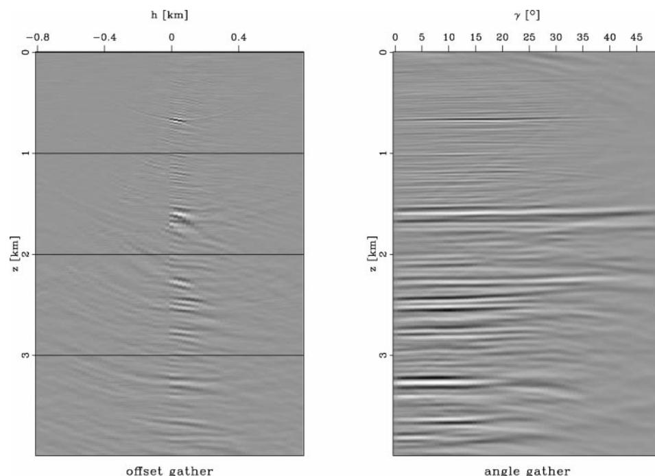
FIG. 14. Three-dimensional common-azimuth example: offset gather (left panel) and angle gather (right panel) corresponding to the vertical line in Figure 13.
