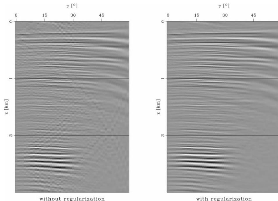
FIG. 12. Two-dimensional real data example: a comparison of an angle gather obtained without regularization (left) and an angle gather obtained with regularization (right).
