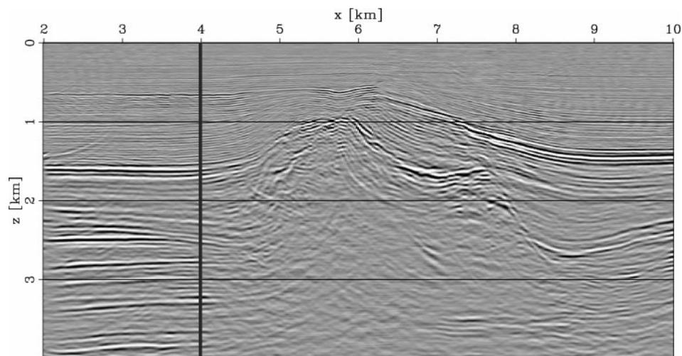
FIG. 13. Three-dimensional common-azimuth example: seismic section obtained by imaging at zero time and zero offset. The vertical line corresponds to the in figure 14.
