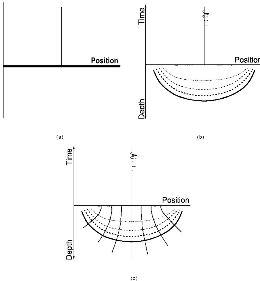
**Figure 1** Propagating isochron: (a) isochron for the minimum two-way traveltime (solid blue line), (b) isochrons for increasing two-way traveltime (the smaller the traveltime, the tinier the dashed line) (c) isochron rays (solid red lines).
