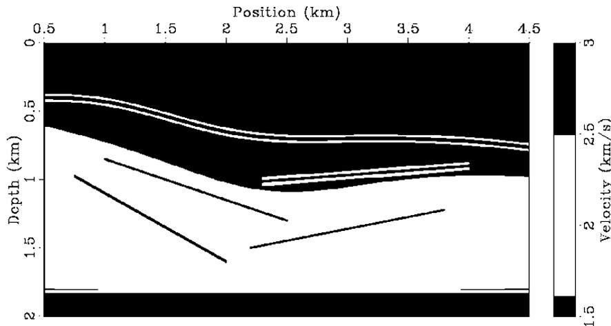
Figure 4 2D seismic model showing the superposition of interfaces and the velocity field.
