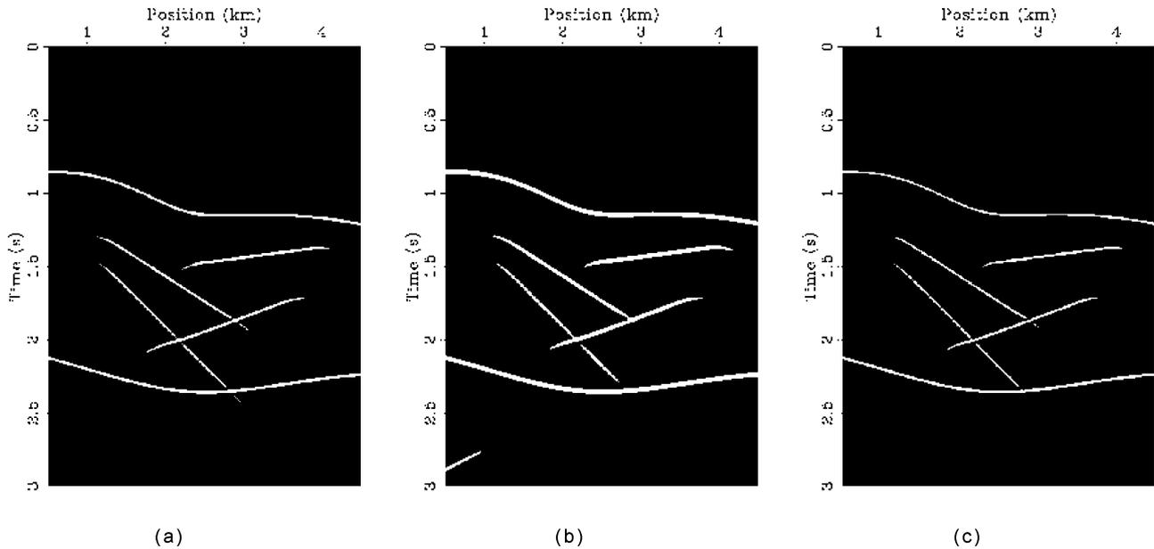
**Figure 5** Common-offset gathers: (a) conventional Kirchhoff modelling, (b) isochron-ray finite-difference modelling and (c) isochron-ray wavefield extrapolation modelling.
