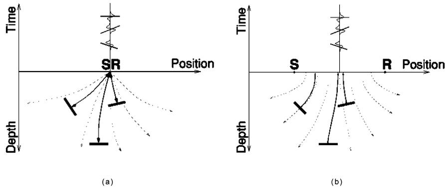
Figure 3 Illustration of data mapping with: a) normal rays and half-velocity for zero-offset data, b) isochron rays and equivalent velocity for common-offset data.
