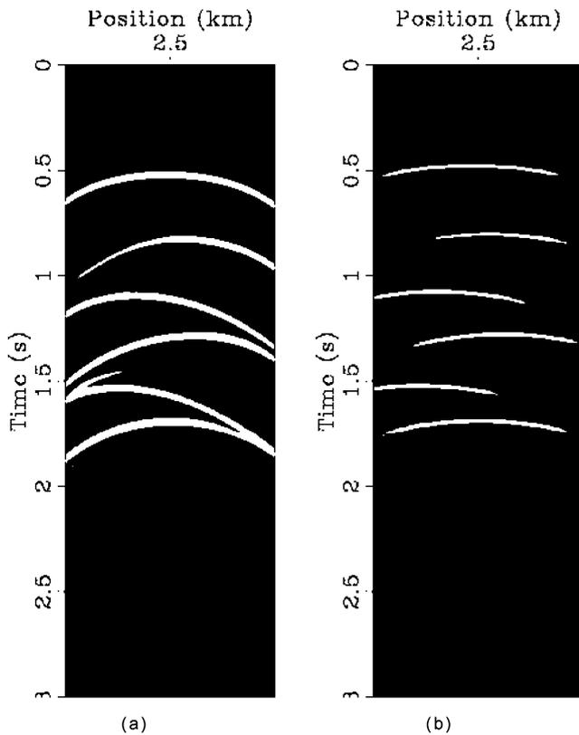
Figure 7 (a) Finite-difference recorded wavefield and (b) extrapolated wavefield recorded at  $z = 5$  m.
