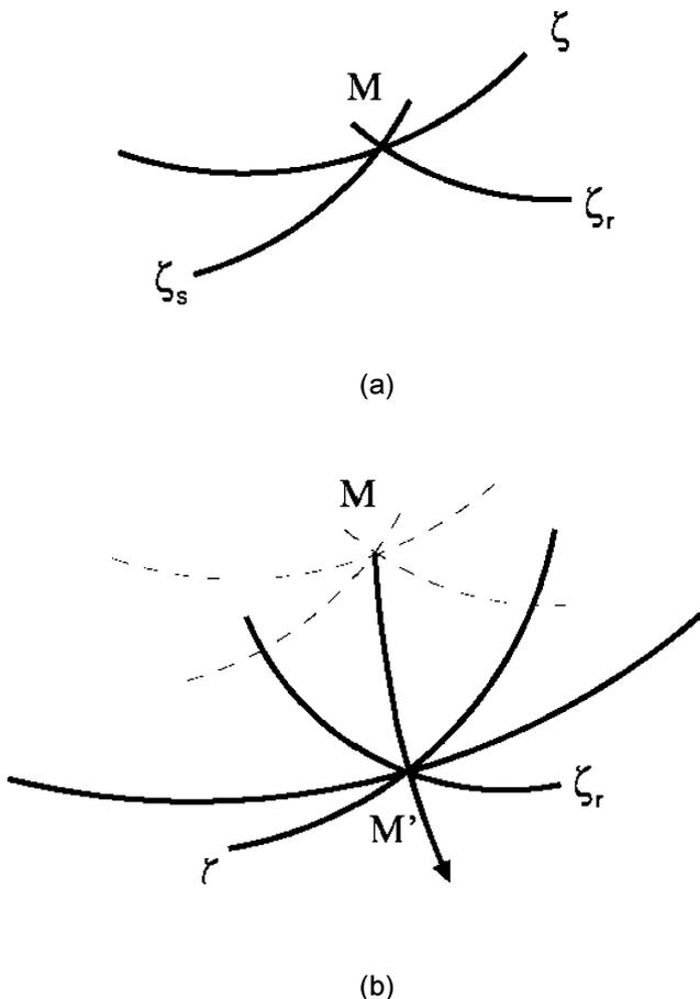
**Figure 2** Isochron ray-tracing scheme: (a) wavefronts at  $t_s$  (blue line) and  $t_r$  (red line), isochron at  $t_r + t_s$  (black line), (b) wavefronts at  $t_s + \delta t/2$  and  $t_r + \delta t/2$ , isochron at  $t_r + t_s + \delta t$ . The isochron ray is the curve determined by the trajectory from  $M$  to  $M'$  (green line).
