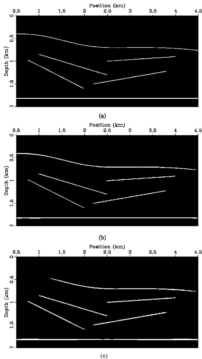
Figure 8 (a) Zero-offset wavefield extrapolation migration, (b) common-offset wavefield extrapolation migration and (c) common-offset reverse time migration.
