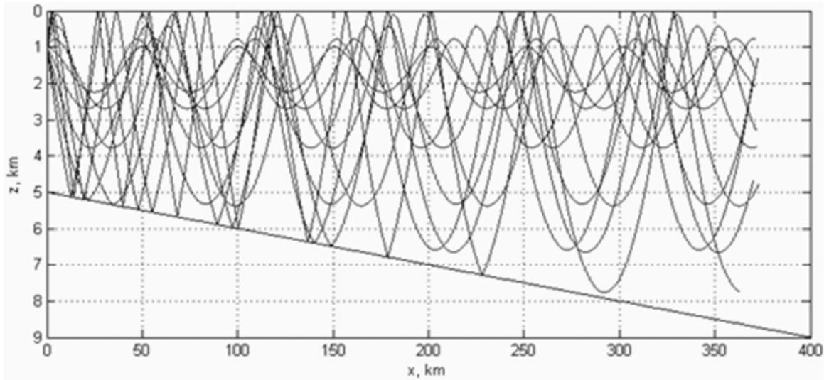
Fig. 5. Ray geometry in the problem of long-range sound propagation in the ocean waveguide with canonical sound speed profile described by Eq. (36) and with two reflecting boundaries ( $z = 0$  and  $z = 5.0 + 0.01x$ , where both  $x$  and  $z$  are expressed in km), obtained with the extended HWT algorithm.
