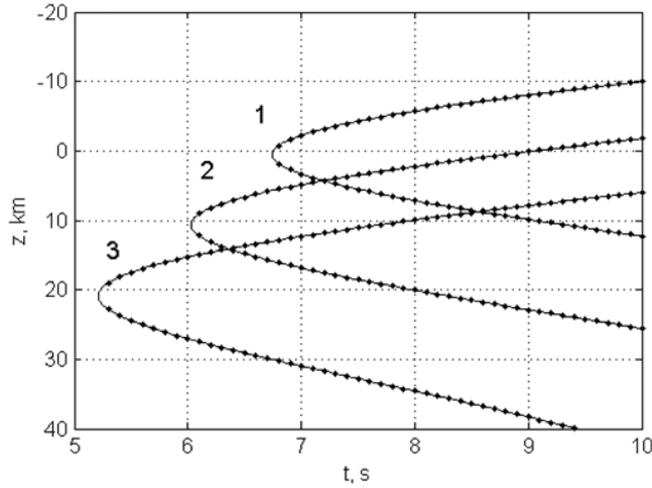
Fig. 2. Timefronts calculated by the extended HWT algorithm (circles) for the model of sound speed  $c(z) = c_0/\sqrt{1-2bz}$  (where  $c_0 = 1.48$  km/s,  $b = 0.01$  km<sup>-1</sup>) and the model of current velocity  $\mathbf{u} = 0$ , compared to analytical solution (22) (lines) for  $x = 10$  km and for the three source locations on the line  $x = 0$ : (1)  $z = 0$ , (2)  $z = 10$  and (3)  $z = 20$  km.
