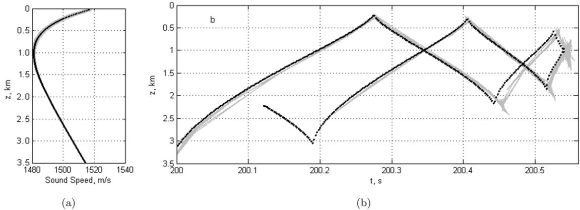
Fig. 6. (a) Sound speed profiles for a model of the ocean waveguide with internal gravity waves at different ranges and range-averaged sound speed profile are shown in grey and black, respectively. (b) Acoustic time-fronts calculated with the extended HWT algorithm for a vertical line array at the range 297 km in an ocean with internal gravity waves (grey) are compared to the time fronts calculated for a range-independent ocean (black). A point source is located at  $x = 0$ ,  $z = 1$  km.
