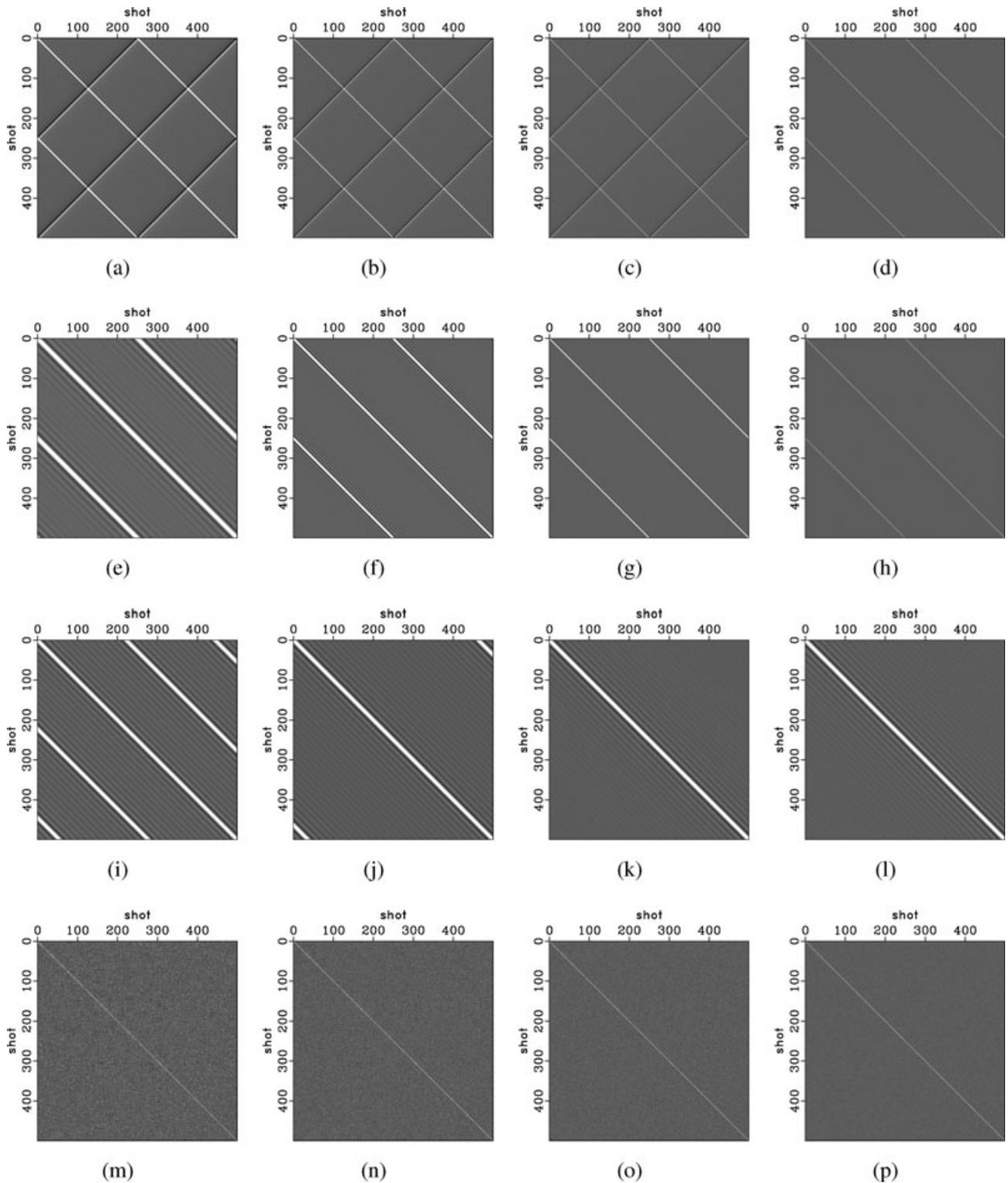
Figure 3 The real part of the crosstalk matrix for 3.0 Hz for the following shot-encoding schemes (top to bottom): Hartley, DFT, plane-wave and random-phase. Each column represents a different number of encodings used with the same shot-encoding scheme from (left to right): 25, 50, 100, 250. All of the crosstalk matrices except those for random-phase encoding have zero imaginary component, which we do not show here for brevity.
