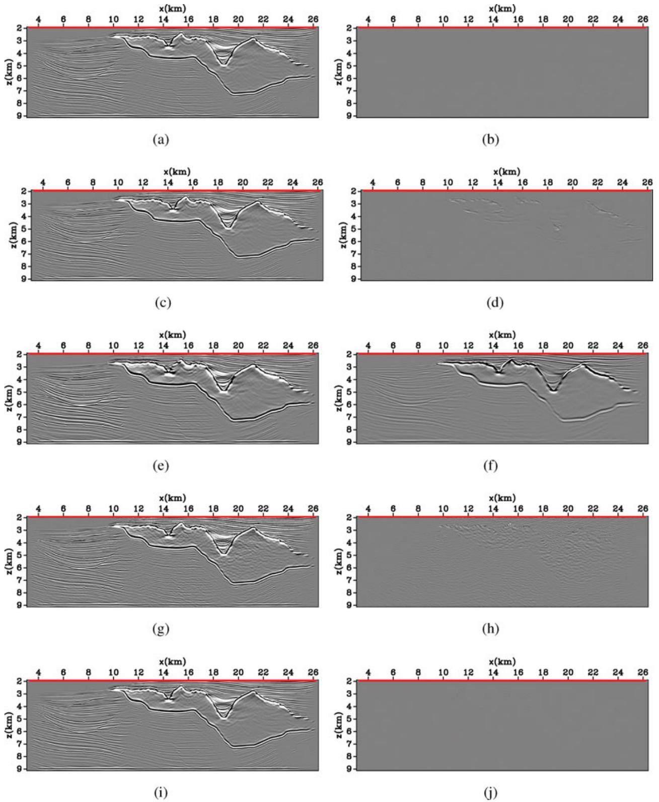
Figure 5 The stacked images (left) and difference images (right) for the following shot-encoding schemes (from top-bottom): Hartley, DFT (modulated-shot), plane-wave, random phase, and decimated shot-record migration. All encodings shown here use 250 encodings.
