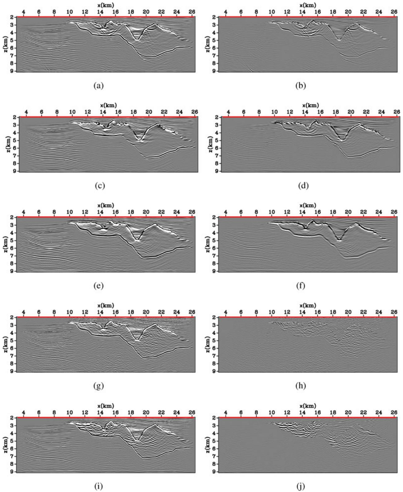
Figure 4 The stacked images (left) and difference images (right) for the following shot-encoding schemes (from top-bottom): Hartley, DFT (modulated-shot), plane-wave, random phase, and decimated shot-record migration. All encodings shown here use 50 encodings.
