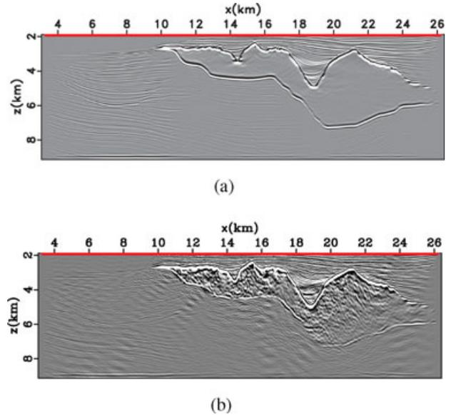
**Figure 1** An example of how crosstalk contaminates the final stacked image for blended images. The (a) image obtained by conventional shot-record migration, (b) is the image obtained by random time-delay encoding, which introduces crosstalk artifacts that severely degrade the quality of the image.
