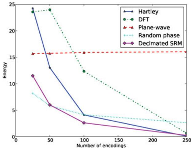
Figure 7 Plots of the energy (lower is better) in the difference image for the various shot-encoding schemes for a group of encodings. The different shot-encodings reconstruct the best quality image at different rates and with different efficiency.
