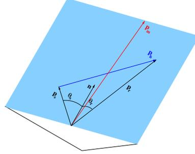
Figure 1: Geometric relations between ray vectors at a reflection point.
