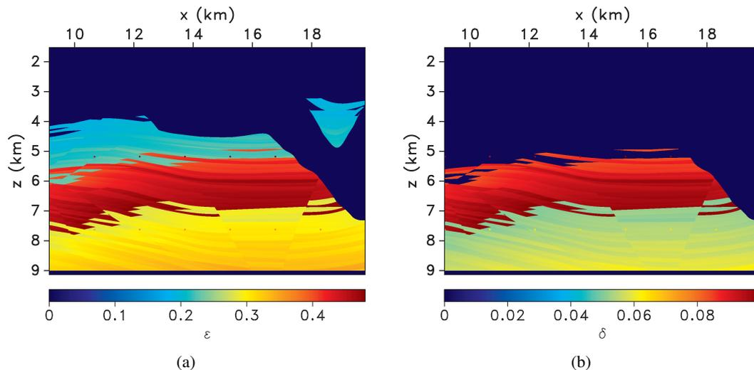
Figure 1: Elastic anisotropic Sigsbee 2A model: (a) parameter  $\epsilon$  ranges from 0 to 0.48 and (b) parameter  $\delta$  ranges 0 from to 0.10.
