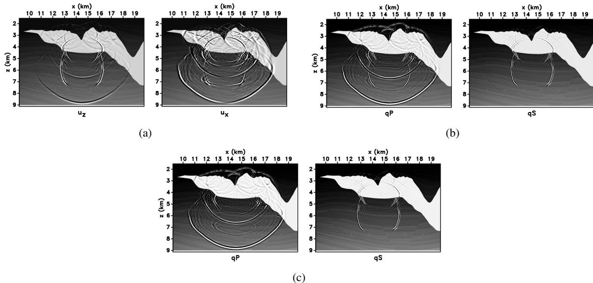
Figure 3: (a) A snapshot of the elastic wavefield. (b) Attempt separation of P and SV modes with  $\nabla \cdot$  and  $\nabla \times$ . (c) Separated P and SV wave modes with anisotropic separators  $\nabla_a \cdot$  and  $\nabla_a \times$ .
