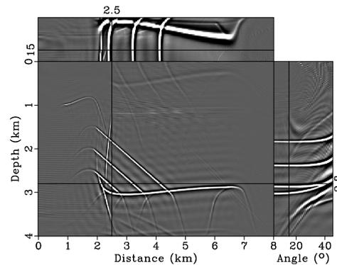
Figure 4: Migrated section after DTI-based migration with velocity of 2 km/s and  $\eta=0.2$  of the TTI synthetic data. The angle gathers obtained, now, using the VTI mapping at 2.5 km location is displayed on the right. The top section shows a depth slice as a function of angle gather at depth 2 km.
