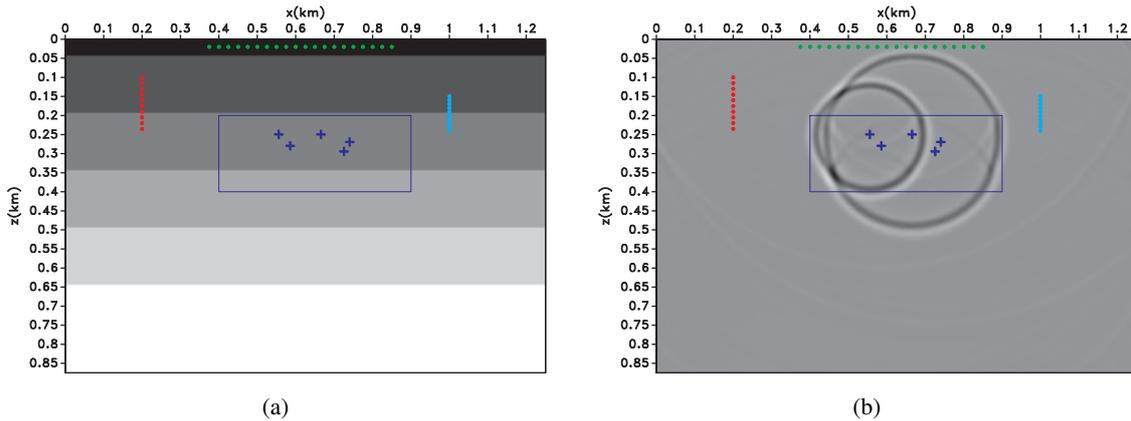
Figure 1: The source and receiver geometry for the synthetic microseismic experiment overlain on the velocity model (a). The receivers are in two boreholes and near the surface. The microseismic hypocenters (crosses) occur randomly in the reservoir of interest at random times over a four second interval as the wavefield snapshot at  $t = 2.65$  seconds shows (b).
