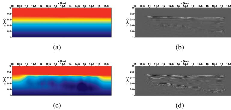
Figure 1: Initial slowness model (a) and corresponding migrated image (b). After 60 iterations, we recover the model in (c); the corresponding migrated image (d) shows improved focusing.
