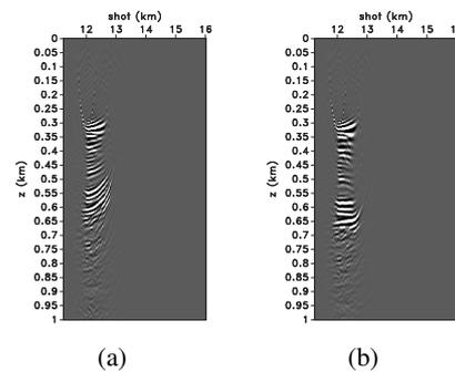
Figure 2: Shot-domain common-image gathers at  $x = 12$  km for the initial model (a) and after inversion (b). The gathers indicate the contribution of each migrated image before stacking.
