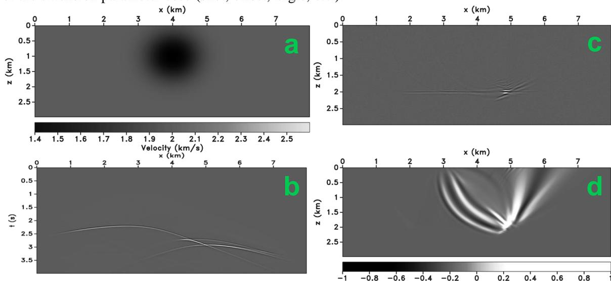
**Figure 1** Migration with a highly refractive model. The velocity model has a strong Gaussian-shaped lens (a) and the reflector is a horizontal density interface at 2km (not shown). Notice the wavefront triplications in the data (b). Migration of a single shot with the correct model gives the image in (c). Notice the spurious artefacts at  $x=5$ km. Image-warping tomography results are strongly affected by the migration artefacts (d).
