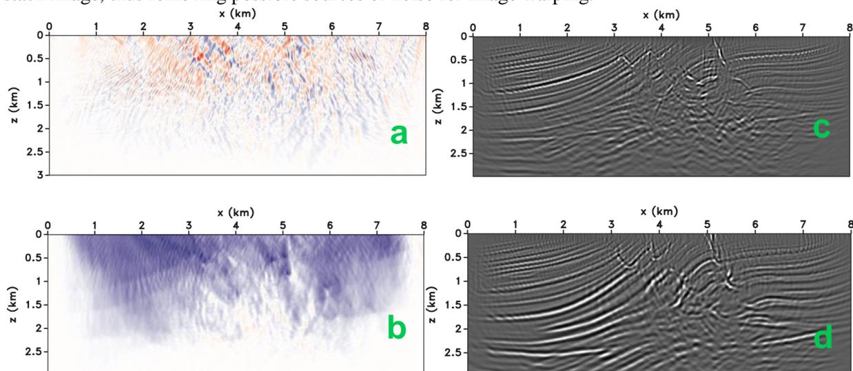
**Figure 2** Marmousi model: first gradient for image domain tomography computed for the image-difference objective function in the shot domain (a) and for the image-warping objective function (b). Migrated images using the initial model (c) and the final model obtained from image-warping tomography (d).
