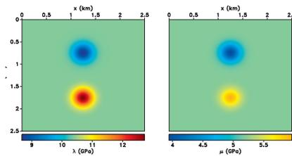
**Figure 1** True  $\lambda$  and  $\mu$  models with a negative and a positive Gaussian anomalies.
