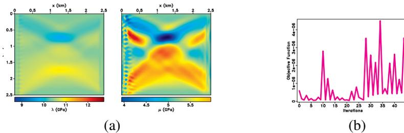
**Figure 2** Example 1: (a) The models recovered with NCG and the (b) inversion objective function.
