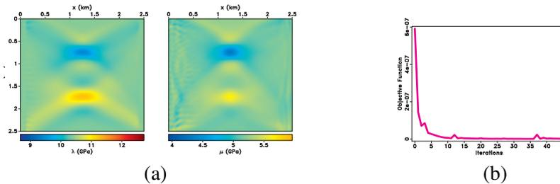
**Figure 3** Example 1: (a) The models recovered with L-BFGS and the (b) inversion objective function.
