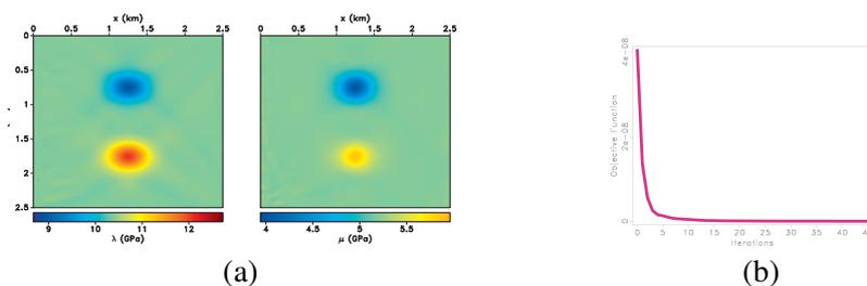
Figure 10 Example 4: (a) The models recovered with L-BFGS and the (b) inversion objective function.
