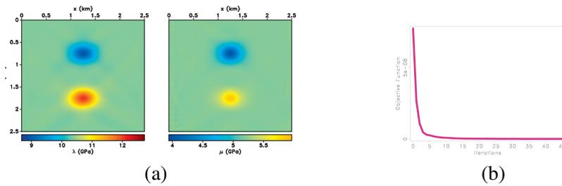
Figure 8 Example 3: (a) The models recovered with L-BFGS and the (b) inversion objective function.
