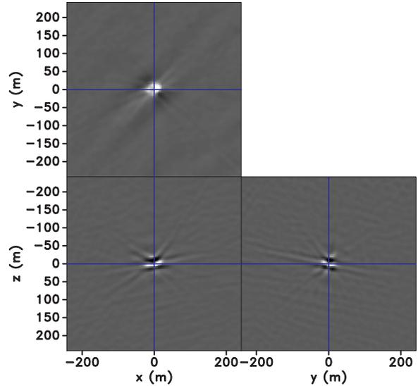
**Figure 5:** Migration PSF for the realistic radar acquisition geometry shown in Figure 2.
