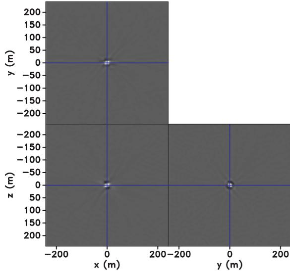
**Figure 3:** Migration PSF for ideal (dense, uniform) radar acquisition at 15 MHz peak frequency.
