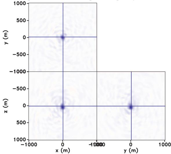
**Figure 4:** Tomography PSF for ideal (dense, uniform) radar acquisition at 5 MHz peak frequency.
