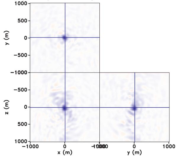
**Figure 6:** Tomography PSF for the realistic radar acquisition geometry shown in Figure 2.
