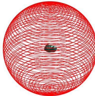
**Figure 2:** Orbital coverage in comet-fixed coordinates after 90 days of continuous radar sounding. The orbiter moves on a sphere of 20km radius.
