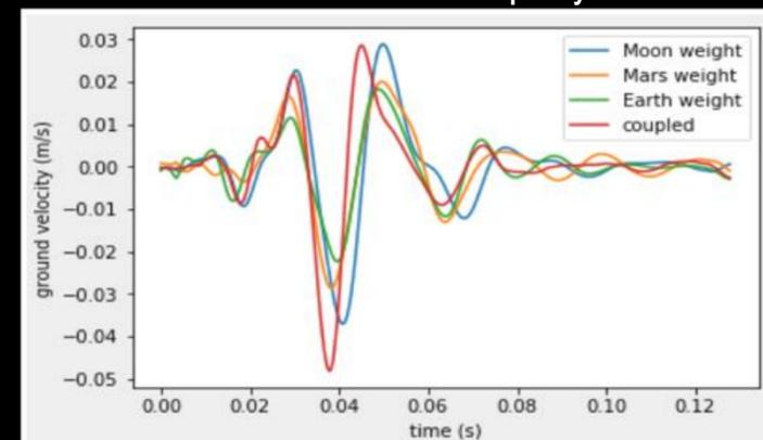
Seismic wave arrival recorded by coupled geophone vs arrival recorded by geophone mounted on 10 kg rover as it would weigh on the Earth, the Moon, and Mars.
