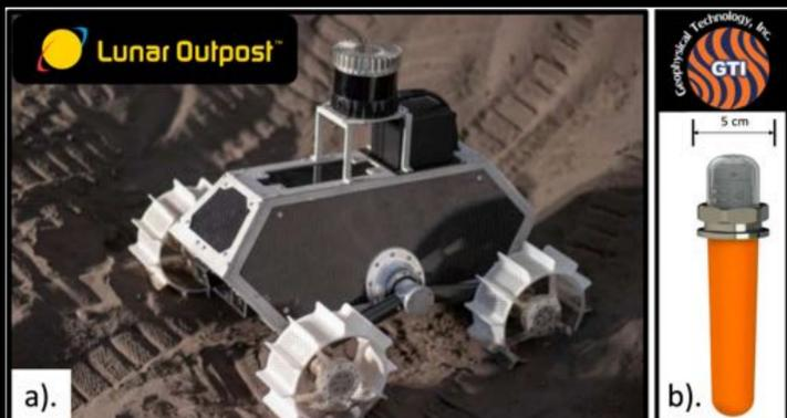
(a) Lunar Outpost's 10 kg autonomous resource prospector rover, ideal for acting as a receiver rover. (b) GTI's NuSeis wireless nodal geophone, ideal for attaching to a small rover.
