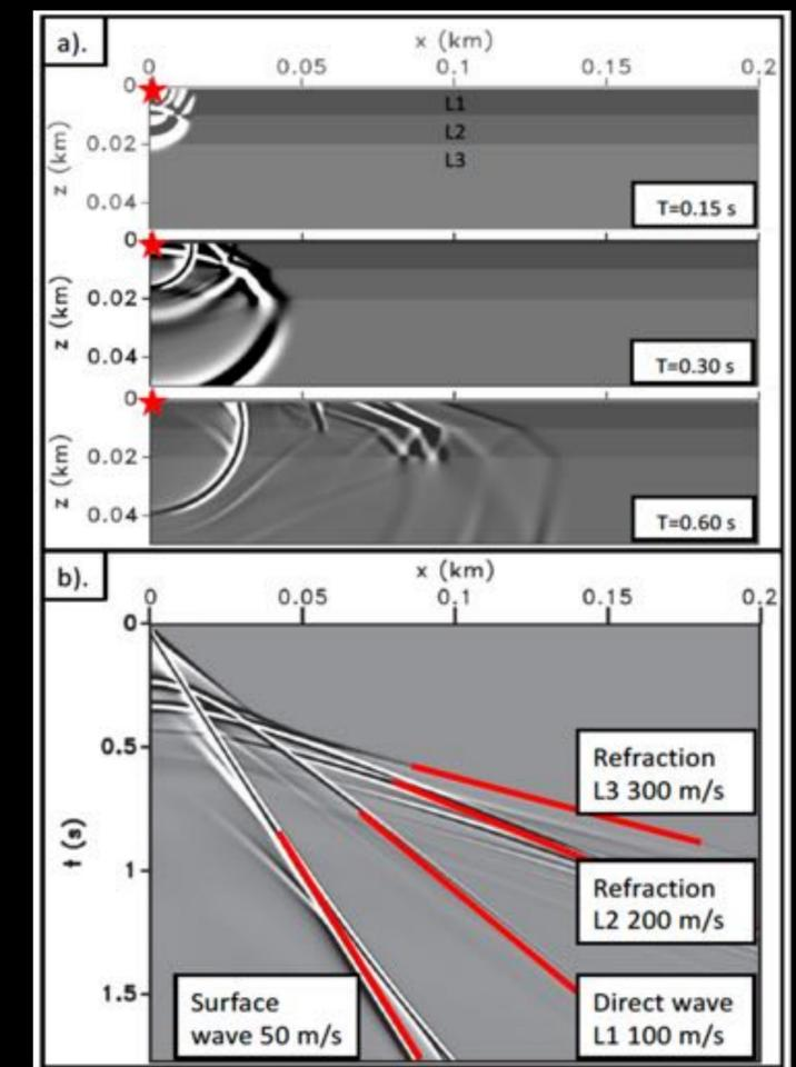
(a) Numerical wavefield simulation of weight drop source over layered regolith model depicted in scenario 1 above. (b) Synthetic data (with interpretation) as would be recorded by ARES along a radial survey line. See abstract for lava tube imaging example
