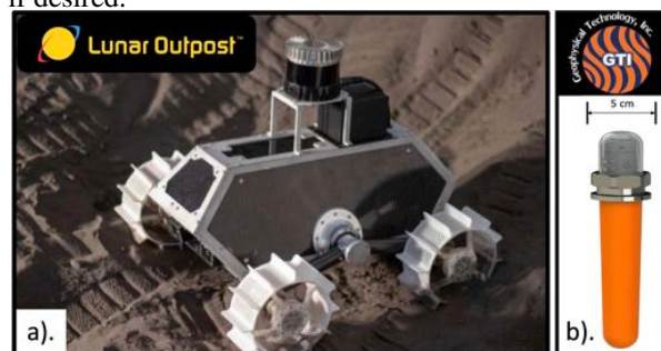
Figure 2: Existing systems for ARES’s receiver rovers: (a) Lunar Outpost’s 10kg Resource Prospector rover ( https://www.lunaroutpost.com ), and (b) GTI’s NuSeis NRU 1C geophone ( https://geophysicaltechnology.com ).
