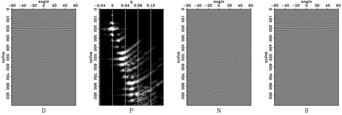
Figure 2: Synthetic example for S/N separation in the image space: (D) data in the image domain; (P) data in the Parabolic Radon domain; (N) multiples (noise); (S) primaries (signal).
