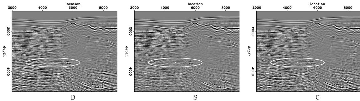
Figure 6: Gulf of Mexico example. Images obtained by angle-domain stacks: (D) signal + multiples (data); (S) primaries (signal) after separation in the image space; (C) primaries (signal) after separation in the data space.
