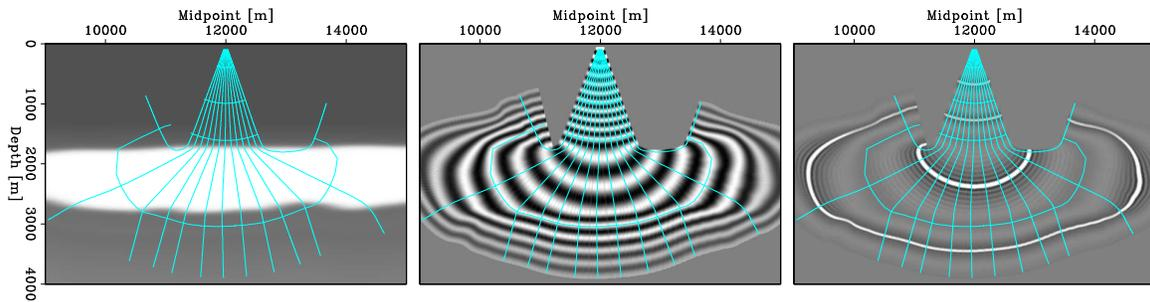
Figure 3: Point source, Gulf of Mexico salt example. Left: velocity model and 5Hz monochromatic rayfield. Middle: 5Hz wavefield. Right: broadband (2-35Hz) wavefield.
