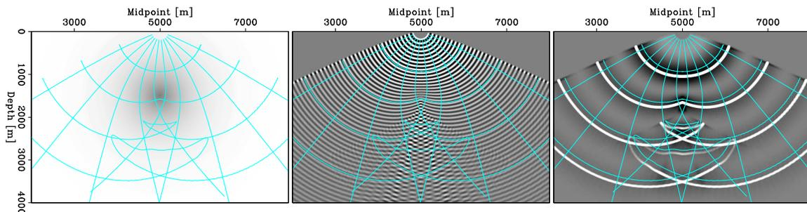
Figure 4: Slow Gaussian slow anomaly example. Left: model with 10Hz coordinate system. Middle: 10Hz wavefield. Right: broadband (0.1-30Hz) wavefield.
