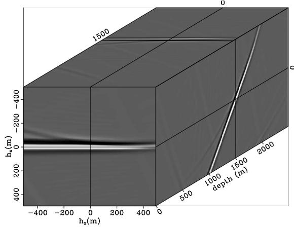
Figure 2: Multi-offset common-image gather for a flat reflector.
