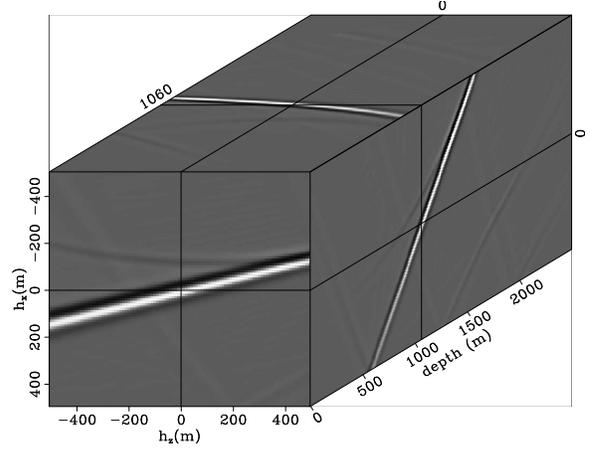
Figure 3: Multi-offset common-image gather for a dipping reflector.
