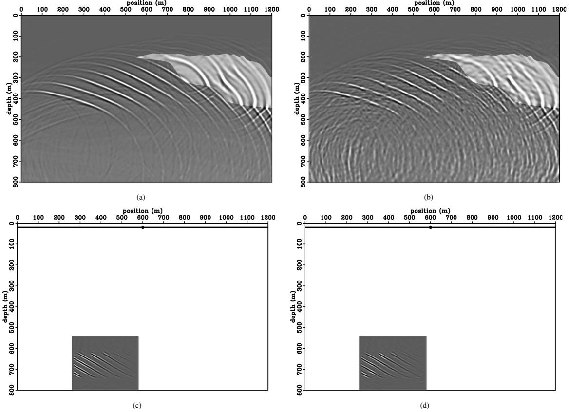
Figure 4: Overlay of reflected wavefield on background velocity model (a) and on velocity model with random variations (b). Image produced by reverse-time migration using the background velocity model for data simulated in the background model (c) and for data simulated in the model with random variations (d). Enlarged images are shown in figures 5(a)-5(d).
