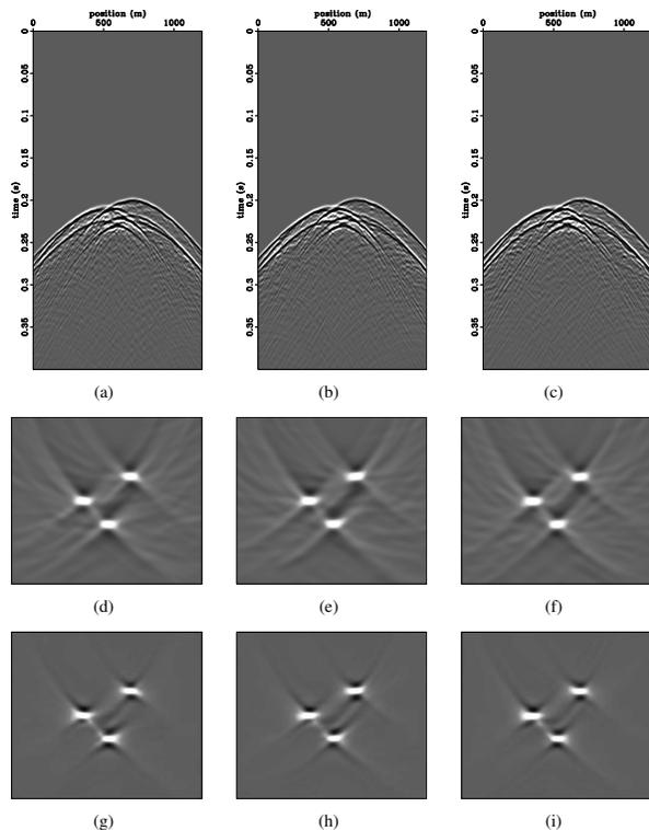
Figure 2: Illustration of statistical stability for the interferometric imaging condition in presence of random model variations. Data modeled with velocity with random variations with magnitude  $\sigma = 20\%$ , for different realizations of the noise model  $n$ . Images obtained by conventional imaging (d)-(f) and images obtained by interferometric imaging (g)-(i).
