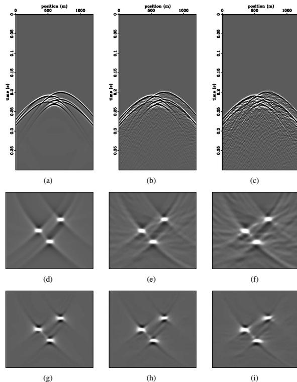
Figure 3: Illustration of interferometric imaging condition robustness in presence of random model variations. Data modeled with velocity with random variations with magnitude  $\sigma = 0\%$  (a),  $\sigma = 15\%$  (b), and  $\sigma = 30\%$  (c). Images obtained by conventional imaging (d)-(f) and images obtained by interferometric imaging (g)-(i).
