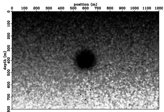
Figure 1: Velocity model with random variations. Imaging targets are 3 point sources located around  $x = 600$  m,  $z = 700$  m.
