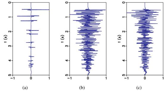
Figure 3: Synthetic seismic data obtained by finite-differences modeling in 1-D models characterized by Figures 1(a)-1(c), respectively.
