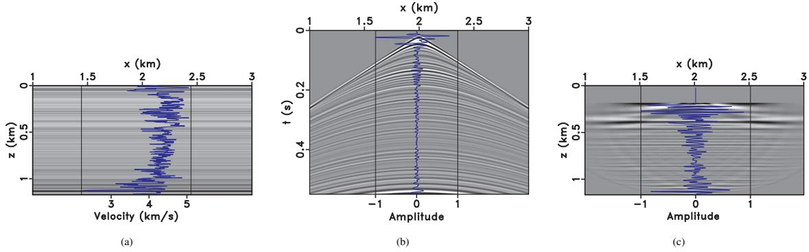
Figure 5: (a) Well-log of P-wave velocity extended horizontally to mimic a subsurface velocity model. (b) Data simulated in a shot-record experiment, with a shot at ( $x = 2.0$  km,  $z = 0$  km); the zero-offset trace is superimposed on the data. (c) Image of the data shown in Figure 5(b) using a conventional imaging condition and a smooth background velocity; the image trace at  $x = 2.0$  km is superimposed on the image.
