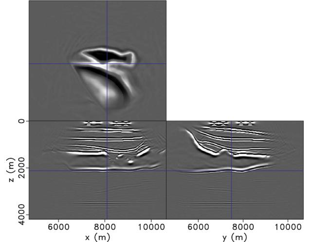
Figure 3: Migrated image for SEG/EAGE salt dome model.
