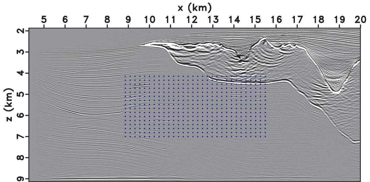
Figure 5: Sigsbee model: shot-record migration of 50 shots. The box highlights the part of the image compared in Figures 6(a)-6(d).
