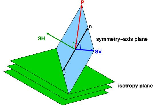
Figure 1: A schematic showing the elastic wave-modes polarization in a 3D VTI medium. Vector  $\mathbf{n}$  indicates the symmetry axis of the TI medium. The P, SV, and SH modes are polarized orthogonal to each other.
