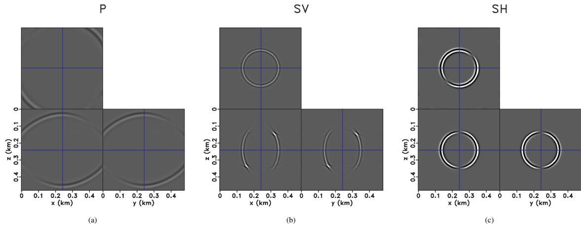
Figure 4: Separated P, SV and SH wave modes for the elastic wavefields shown in Figures 3(a)-3(c). P, SV, and SH are well separated from each other.
