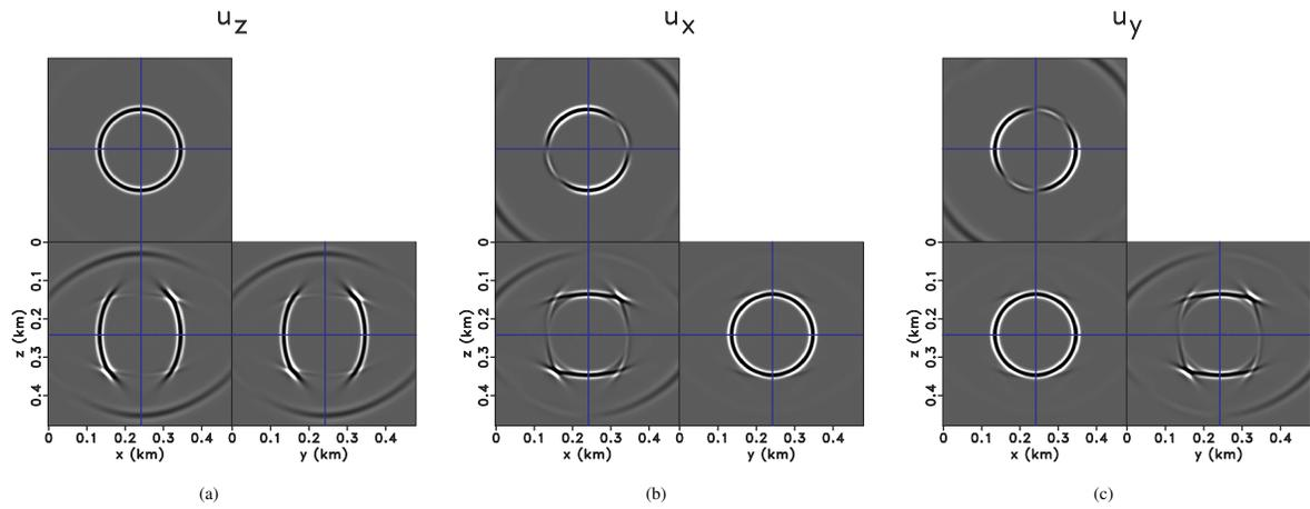
Figure 3: A snapshot of the elastic wavefield in the  $z$ ,  $x$  and  $y$  directions for a 3D VTI model. The model has parameters  $V_{P0} = 3.5$  km/s,  $V_{S0} = 1.75$  km/s,  $\rho = 2.0$  g/cm<sup>3</sup>,  $\varepsilon = 0.4$ ,  $\delta = 0.1$ , and  $\gamma = 0.0$ . A displacement source located at the center of the model oriented at vector direction  $\{1, 1, 1\}$  is used to simulate the wavefield.
