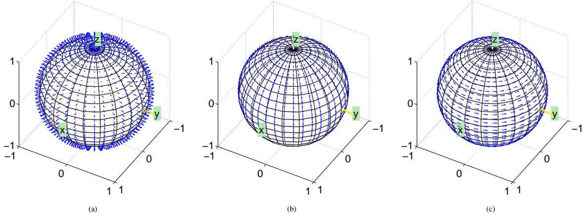
Figure 2: Panels (a) to (c) correspond to the wave-mode polarization for P, SV, and SH mode for a VTI medium obtained using Equations 6 and 7. Note that the SV and SH wave polarization vectors have zero amplitude in the symmetry axis direction.
