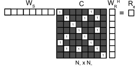
Figure 1: In blended source imaging, the  $R_e$  image is the original image plus additional artifacts from the cross-talk or the off-diagonal terms in  $C$ . When the cross-talk matrix  $C$  is the identity matrix  $I$ , then the product of  $W_S$ ,  $C$  and  $W_R^H$  represents conventional seismic imaging and  $R_e$  becomes the conventional image  $R$ .
