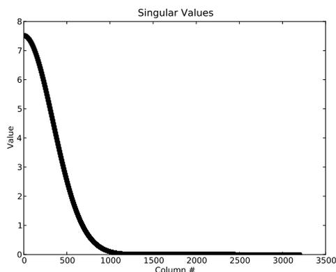
Figure 3: The singular values from the decomposition of the cross-talk matrix with the Gaussian approximation to the identity matrix. Since singular values close to zero do not contribute to the image, the best possible image for the Gaussian approximation is constructed for 1000 singular values (experiments).
