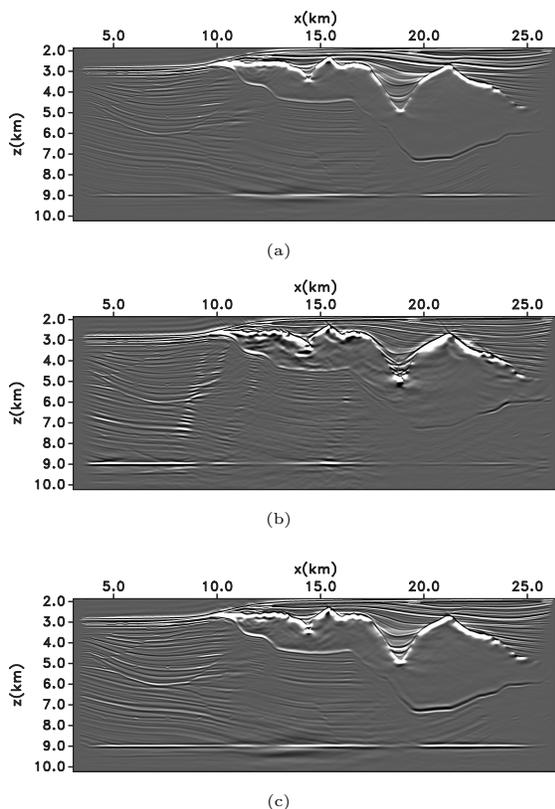
Figure 4: The image of Sigsbee using the conventional shot-record migration (a), the Gaussian approximation to the identity matrix for 10 blended experiments (b), and 100 blended experiments (c).
