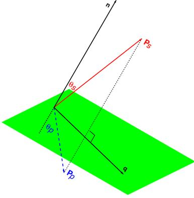
Figure 1: A cartoon illustrating a P to S reflection upon a reflector. The reflection plane and the reflector intersect along a line defined by the vector  $\mathbf{q}$ . The reflector has a normal defined by the vector  $\mathbf{n}$ . The source and receiver rays are characterized by the vectors  $\mathbf{p}_p$  and  $\mathbf{p}_s$ , respectively. The incidence and reflection angles are denoted by  $\theta_p$  and  $\theta_s$ , respectively.
