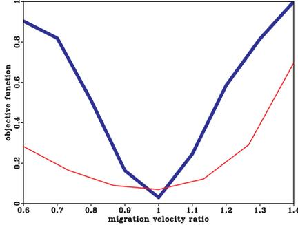
Figure 6: Objective function for PP and PS CIGs by applying the penalty functions, Figure 5(e) and (f), to PP and PS CIG gathers respectively. The thick line is for PP data, and the thin line is for PS data. The horizontal axis is the ratio of migration velocity and true model velocity. The PS CIG gathers are obtained using correct P-wave velocity.
