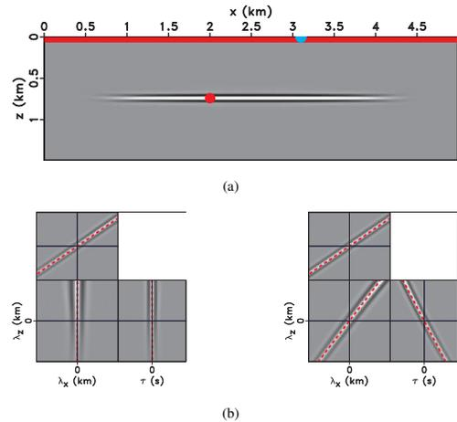
Figure 2: (a) The experiment geometry used to construct the CIP gathers in panel (b). The dot on the surface represents the shot location, the line on the surface represents the receivers, and the dot on the reflector represents the CIP location. A common image point reflection for PP (left) and PS (right) data for the experiment shown in Figure 2(a). The overlain dashed line is given by equation 9 and matches exactly with the CIP reflection moveout.
