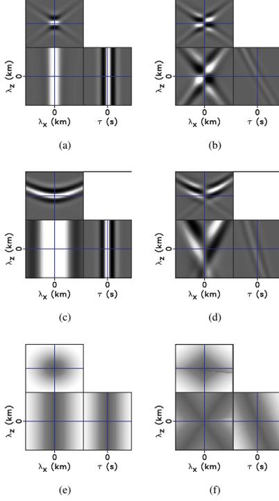
Figure 5: Panels (a) and (b) show CIG gathers for PP and PS data, respectively, obtained with correct velocity. Panels (c) and (d) are the PP and PS CIG gathers for incorrect velocities. The (e) PP and (f) PS penalty functions are given by equations 16 and 19, respectively.
